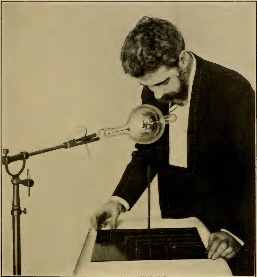
PLATE 53.—Author's Position Finder. Ready method of centring plate with focus of tube, as taught in the text. Operator is sighting down anode and along rod to base. The lines on the base show different sizes of photographic plates, each of which has a centred hole for the rod. Shift the base with the hands till the focus is sighted, then remove the rod and lay the plate on the base film side up. Then place the part to be radiographed on the plate with its marked centre on the centre of the light-proof wrappers. See text for full directions.
